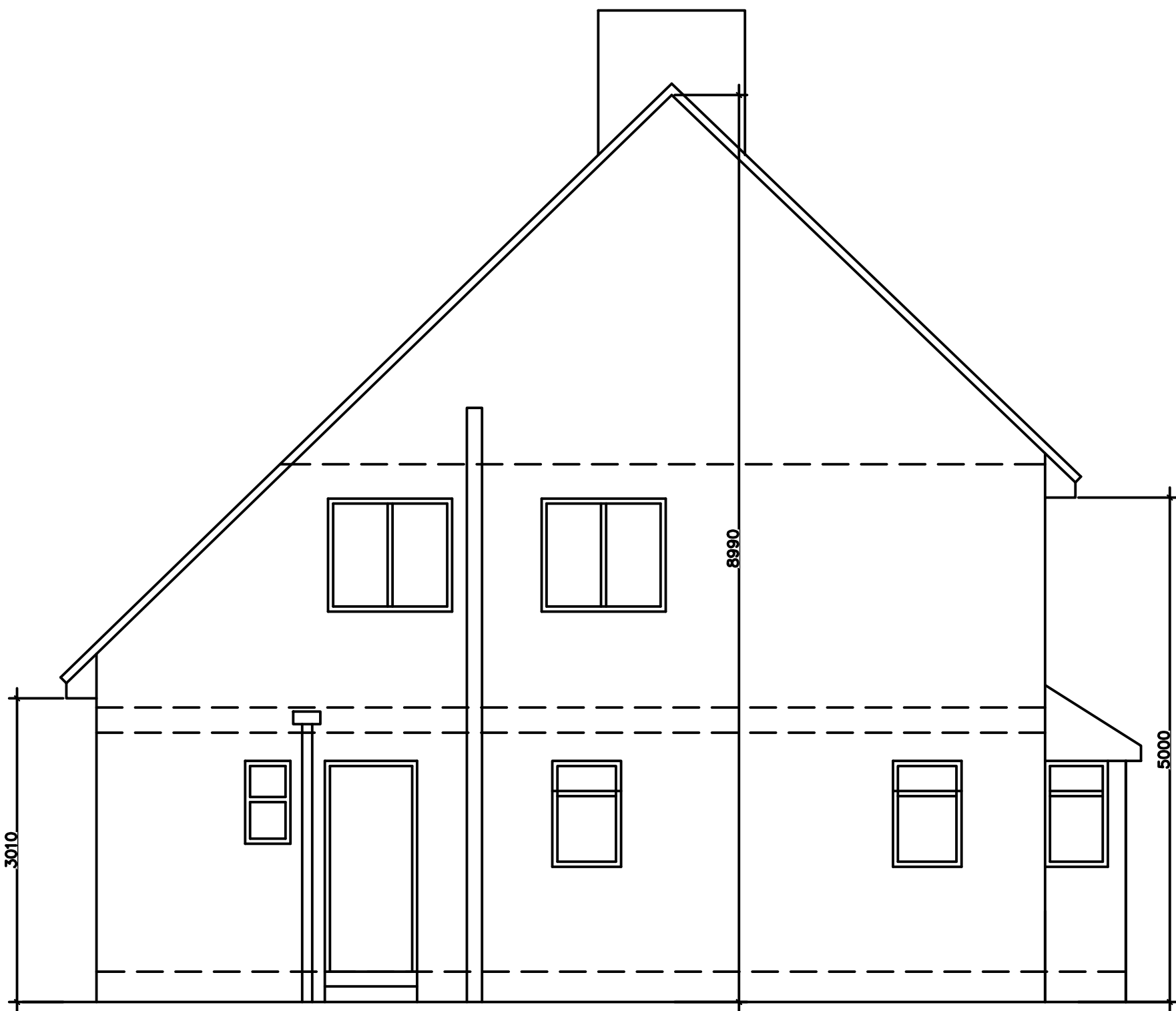
EXISTING SIDE ELEVATION
